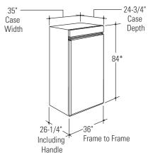
\*Shipped at 84" installation height. Can be adjusted to 83-1/2" or 84-1/2" with Grille Panel Kits.
